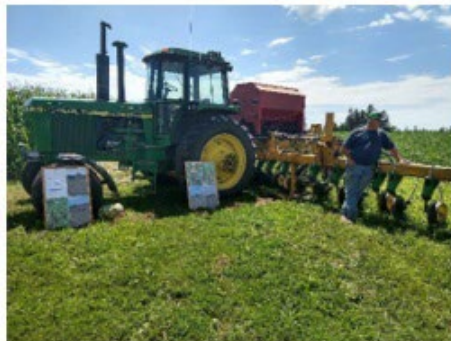
Pictures to left is Mark Stock with his custom air seeder. It was constructed from a Gandy air seeder box and a cultivator tool bar with single disc fertilizer openers.
