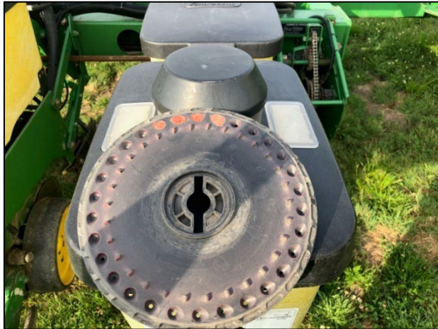
Image 1. Seed spaces blocked on wheel to plant corn with 'skip rows.'
