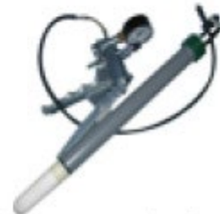
Soil Suction Sampler (ACM-SSS-2676)
