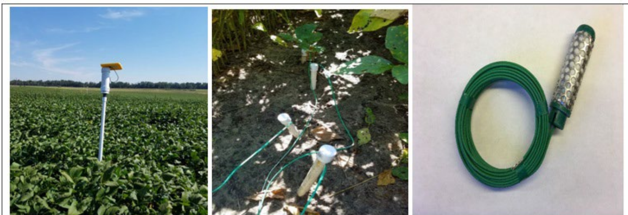
Figure.1. Watermark sensors and mounting pole installed in the grower's demonstration fields with cellular data transmitter and solar panel.
