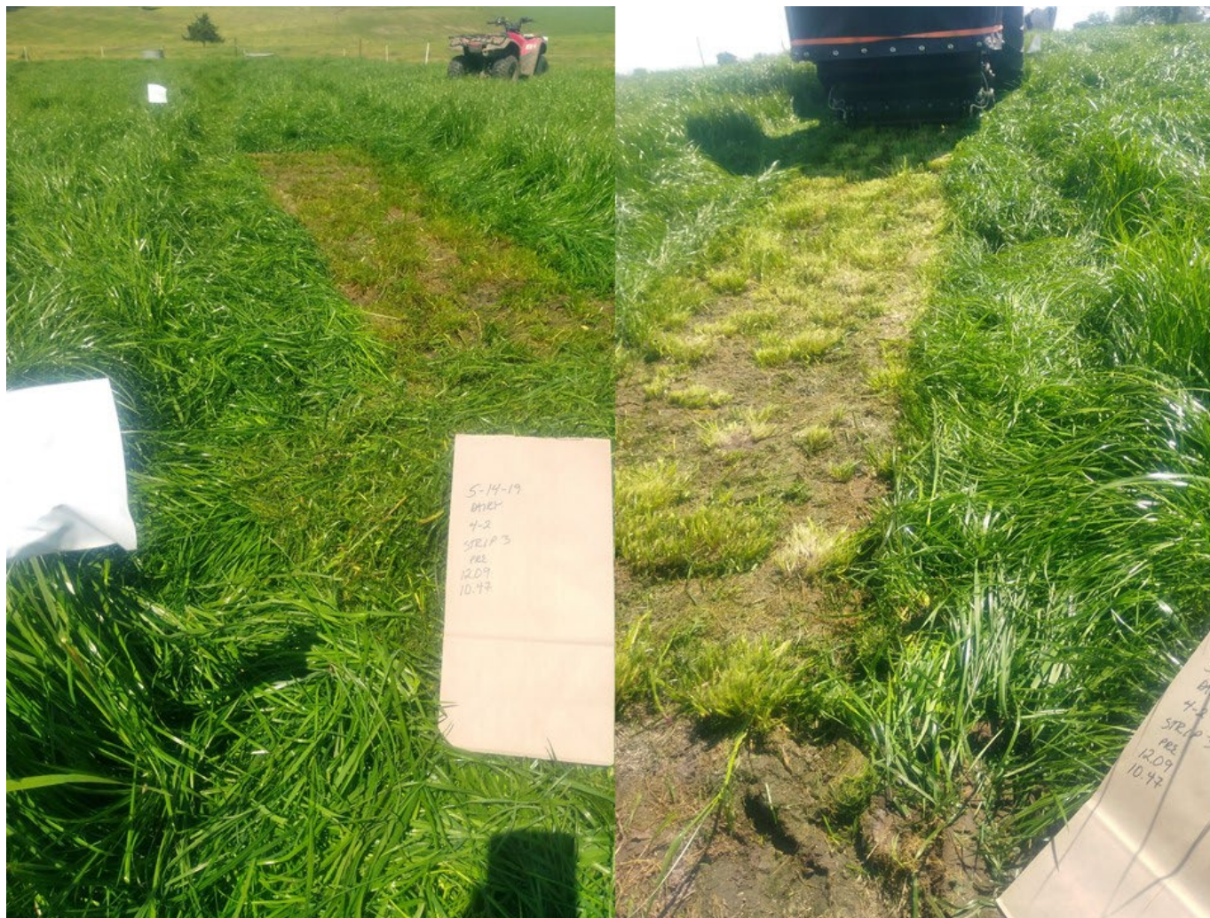
Figure 10. Field work to determine relationship between forage height and mass in Perennial ryegrass. This species is less common on traditional farms across Missouri but renovated grasslands use it more frequently. The left panel shows a cut strip that was measured by the ultrasonic sensor on the ATV before and after harvesting (right panel). Samples are retained for dry matter to develop relationships between forage height and forage yield.
