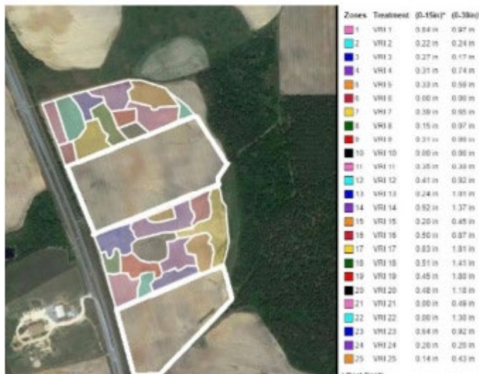
Figure 3: Resulting variable prescription map, with alternate uniform irrigation application zones.
