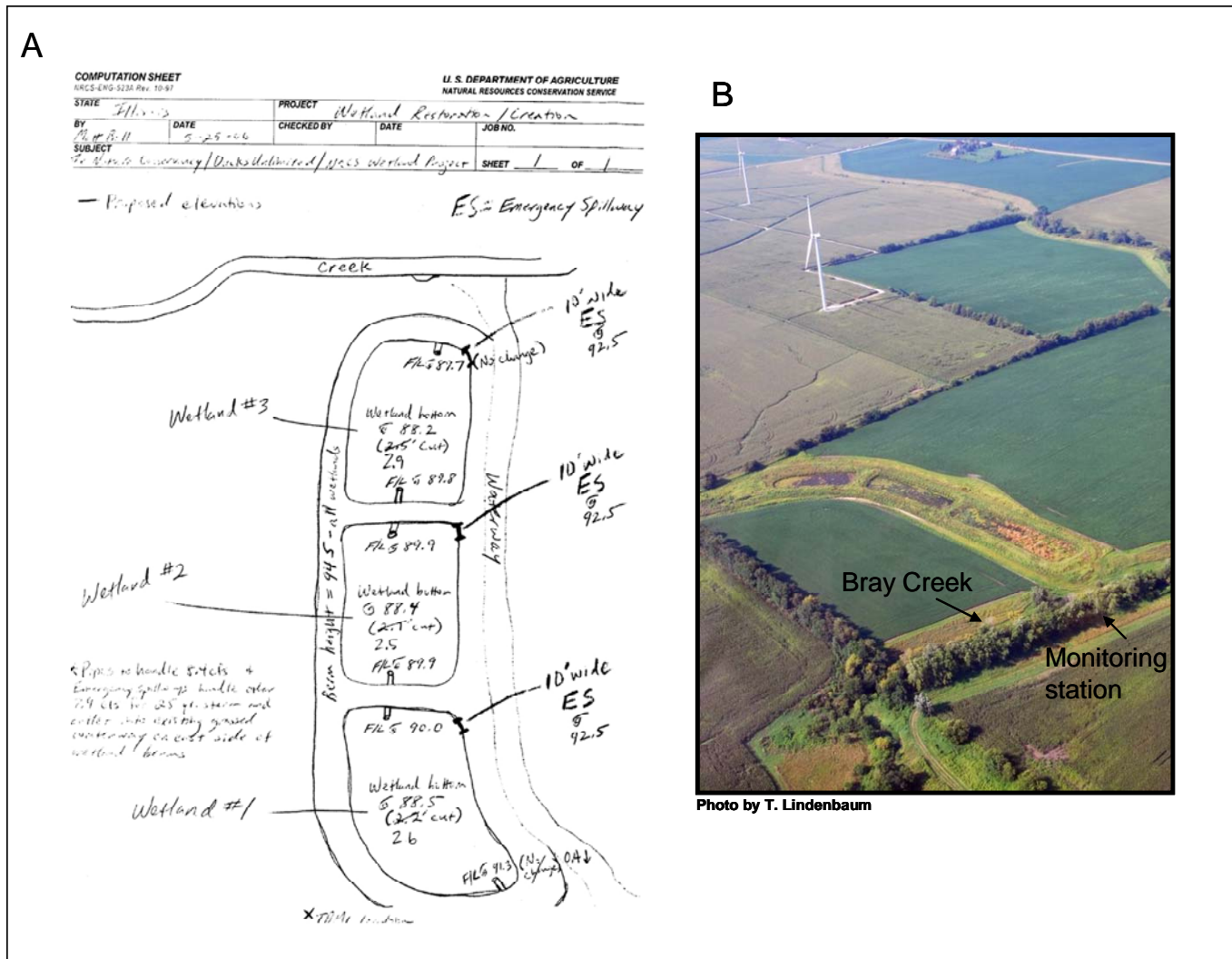
Figure 3. Detailed map showing the upstream wetland site design (A) and aerial view (B) photographed August 2008.
