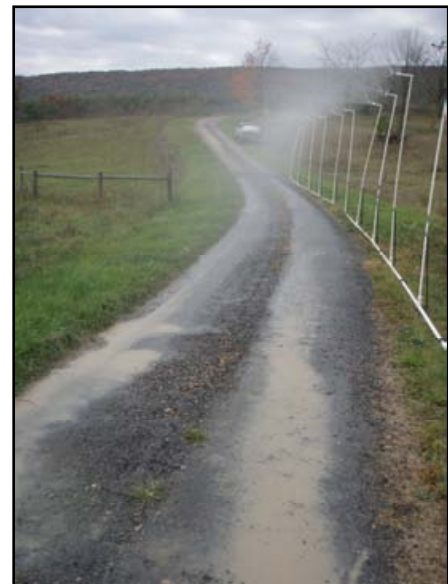
Figure A4: The rainfall simulator being run on Pruss Lane in Mifflin County.
