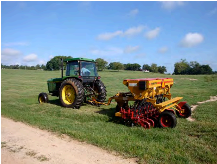
Demonstration of no-till grain drill for dairy producers. Drill was provided through partnership with Oconee River RC&D Council.
