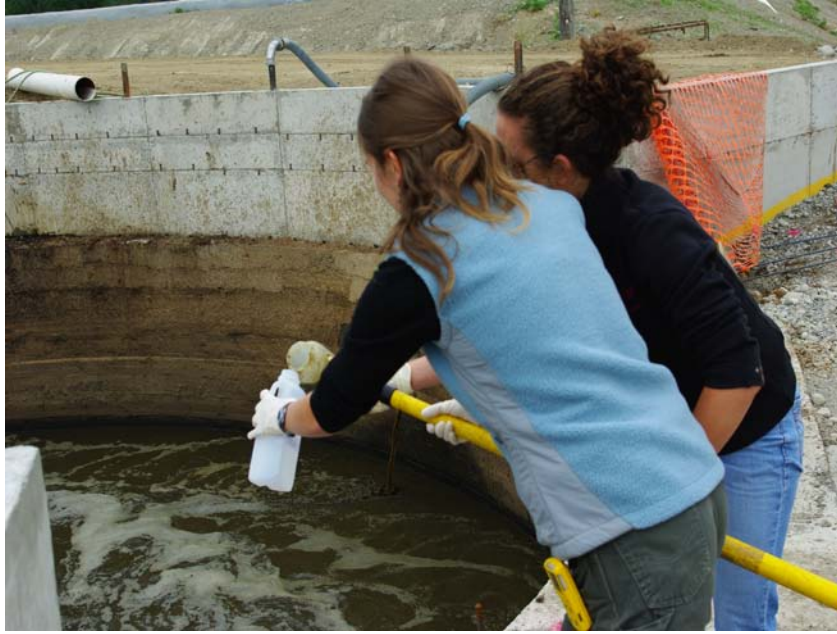
Figure 13. Sampling incoming manure and pre-consumer food-wastes at the receiving tank
