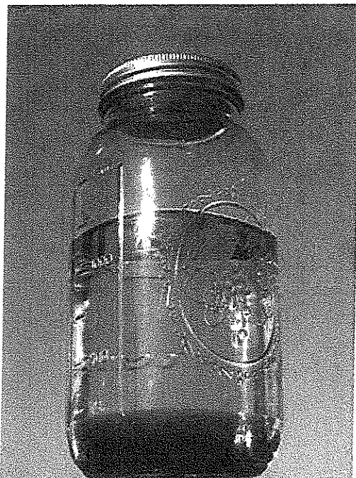
Figure 2 Light-colored biodiesel is on the top and dark colored glycerol is settled at the bottom of the jar
