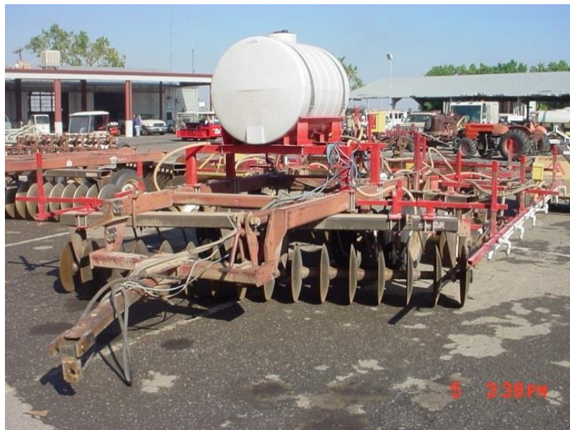
Figure 5. The disk and the mounted dust control unit.
