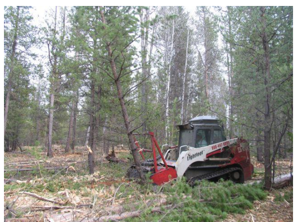
Photo 6. Mastication of lodgepole pine at Westfall demo site.
