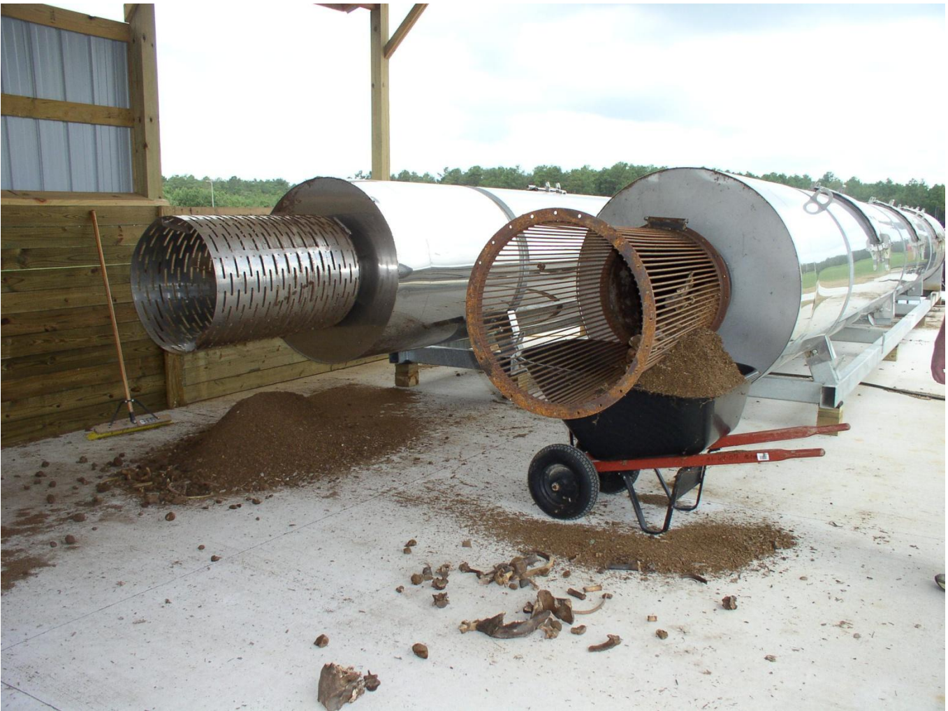
Figure 3: Biovator rotary composters on the Henry Moore Farm.
