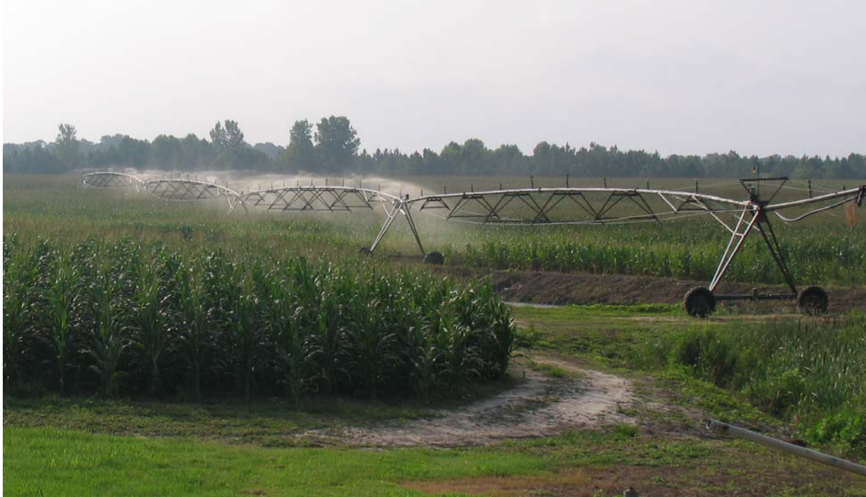
Figure 4. CP with VRI controls turning off certain sprinklers as sensitive areas are passed.
