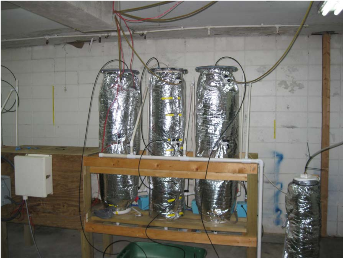
Figure 6. Pilot scale anaerobic digesters like the ones above were installed at the lagoon site, with some problems. The ones shown above are operated at the SADAEL in Tifton, GA to monitor gas production from fruit and vegetable waste and animal waste.
