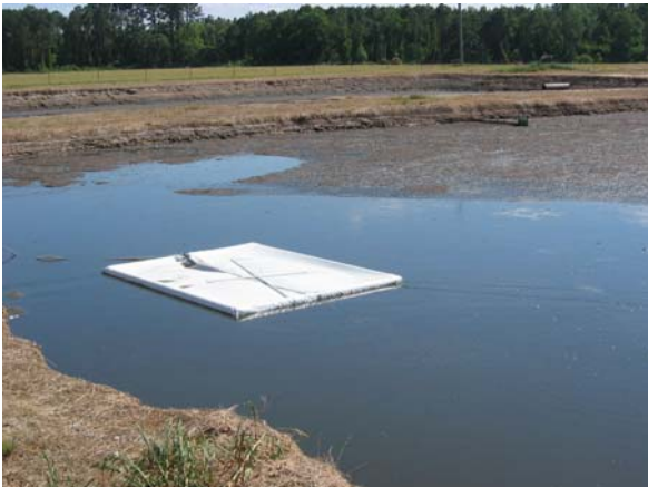
Figure 12. A test floating cover to determine the quantity of biogas that could be produced in a poultry lagoon system.
