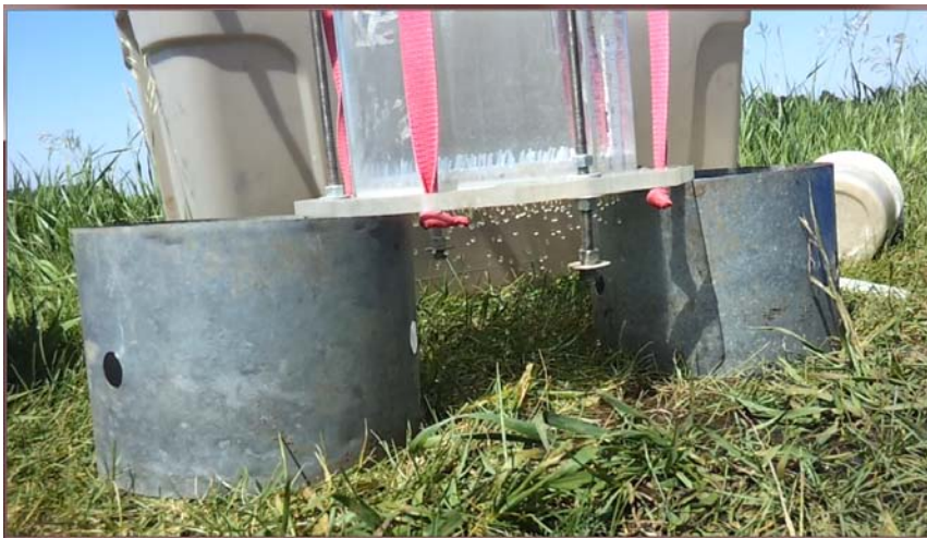
Figure 4. Rainfall pattern from a Cornell sprinkle infiltrometer.
