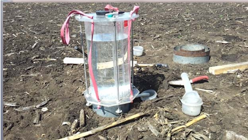
Figure 3. Cornell sprinkle infiltrometer field set up.
