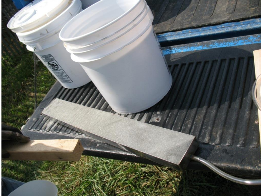
Figure 5: Lysimeter Pan Filled with Glass Beads
