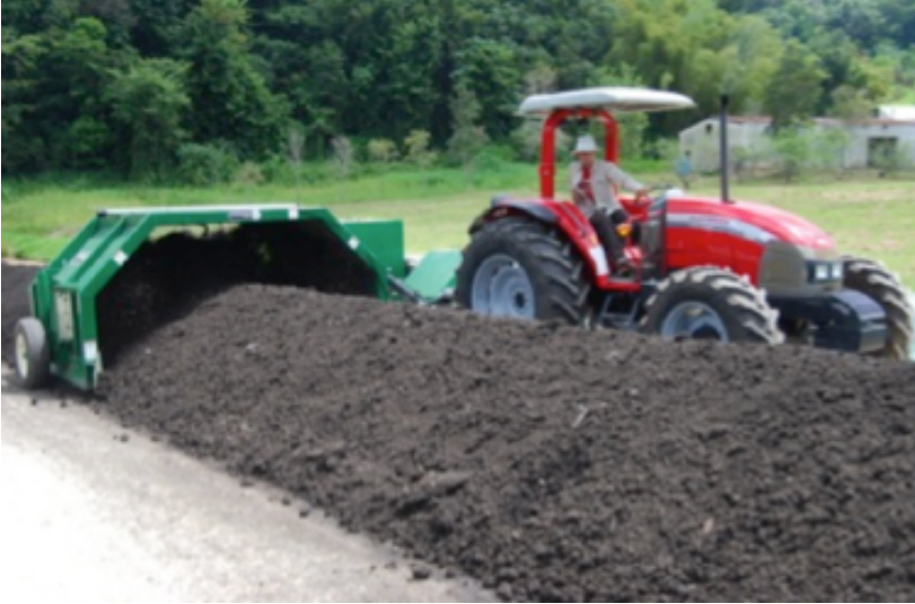
Image 4. Aeromaster PT-120 pull type-windrow turner pulled by a McCormick C105 max 99hp tractor
