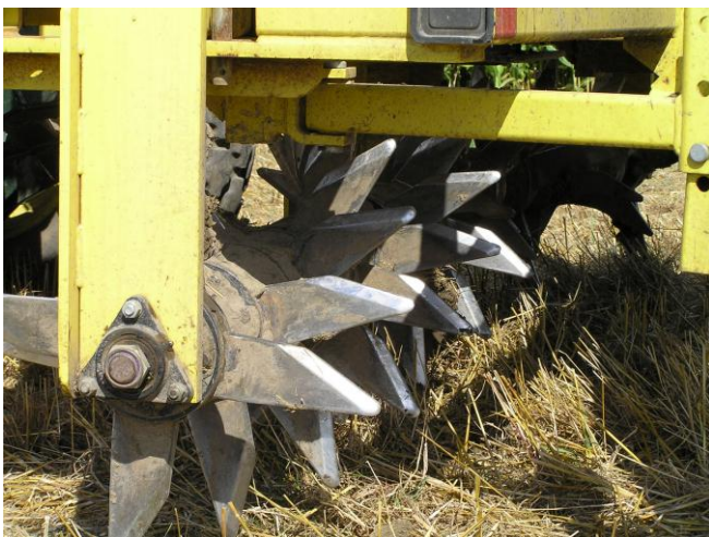
Figure 2. Aeration tines loosen and fracture the soil and improve infiltration with little loss of crop residues.
