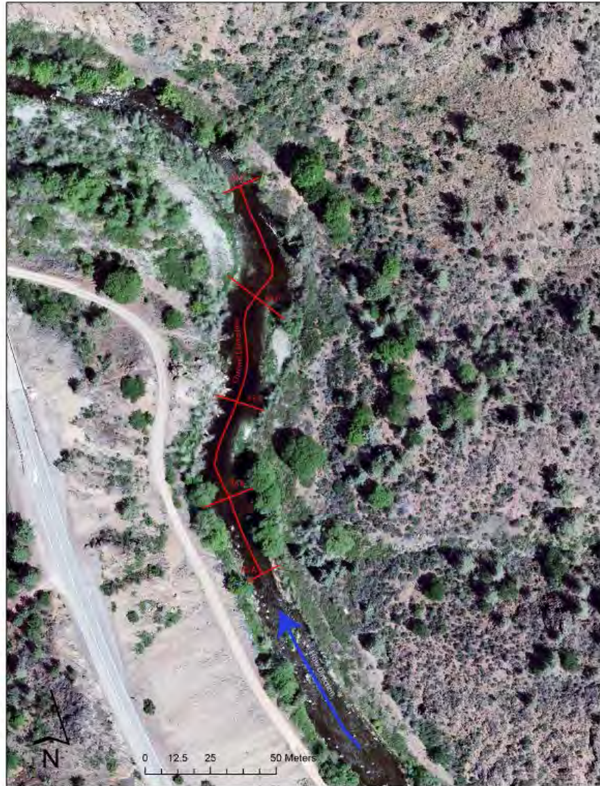
Figure A-4. Spatial layout of cross-section surveys within a pool.
