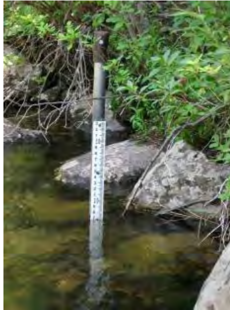
Figure B-1. An example of a continuous stage recorder deployed with a pipe housing and staff gauge.
