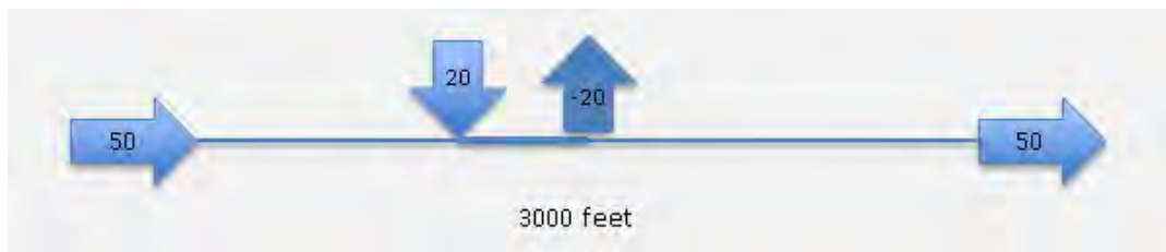
Figure 1 - Reach schematic of the model used for testing various input parameters.
