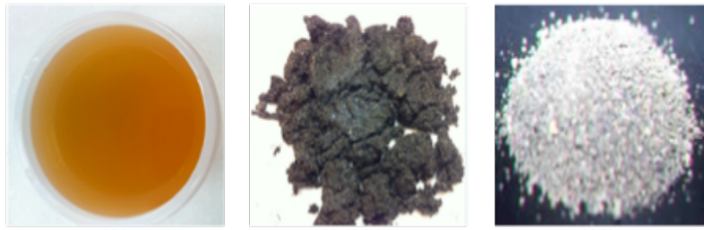
Figure 4. Nutrient recovery products including (left to right) bio-ammonium sulfate solution, phosphorus-rich solids and phosphorus containing struvite crystals.
