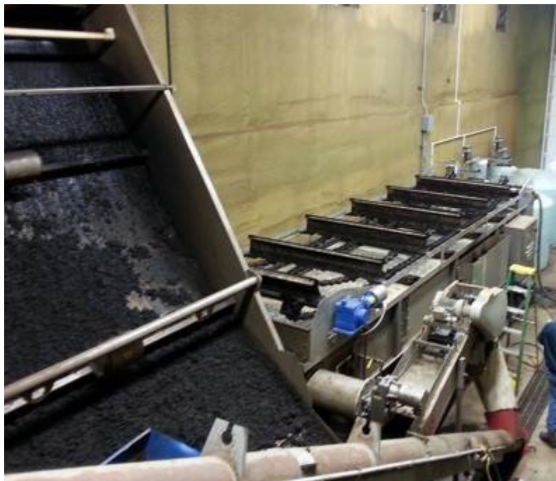
Figure 3. Commercial-scale recovery of P solids, integrated with dairy anaerobic digester in Bio-Town, IN (AD facility is not shown in photo).
