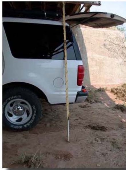
Figure 11: Example of a differential-pressure transducer. Note the cable extended above the transducer on the wooden lath.
