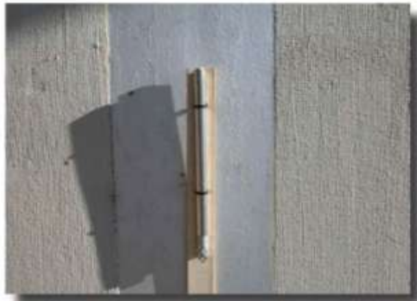
Figure 12: Absolute pressure transducer attached to a wooden lath and secured with nylon ties.
