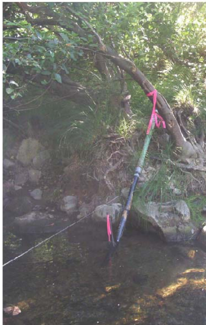
Figure 14: Pressure transducer in plastic pipe housing
