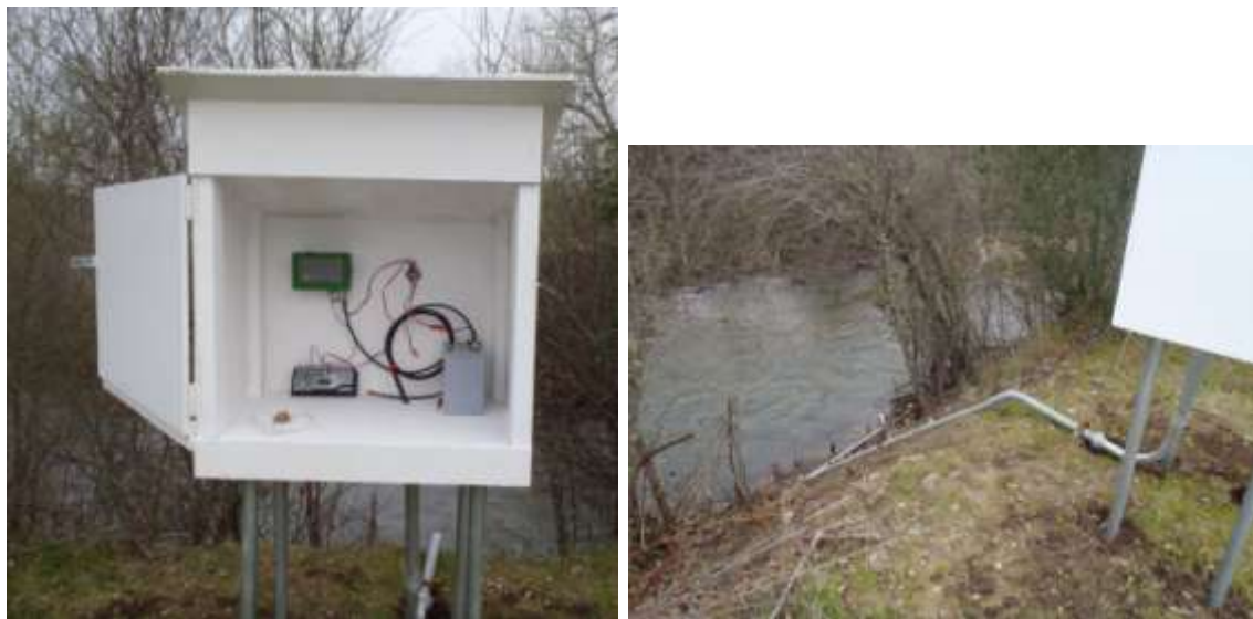
Figure 10: Bubble system type stream gage
