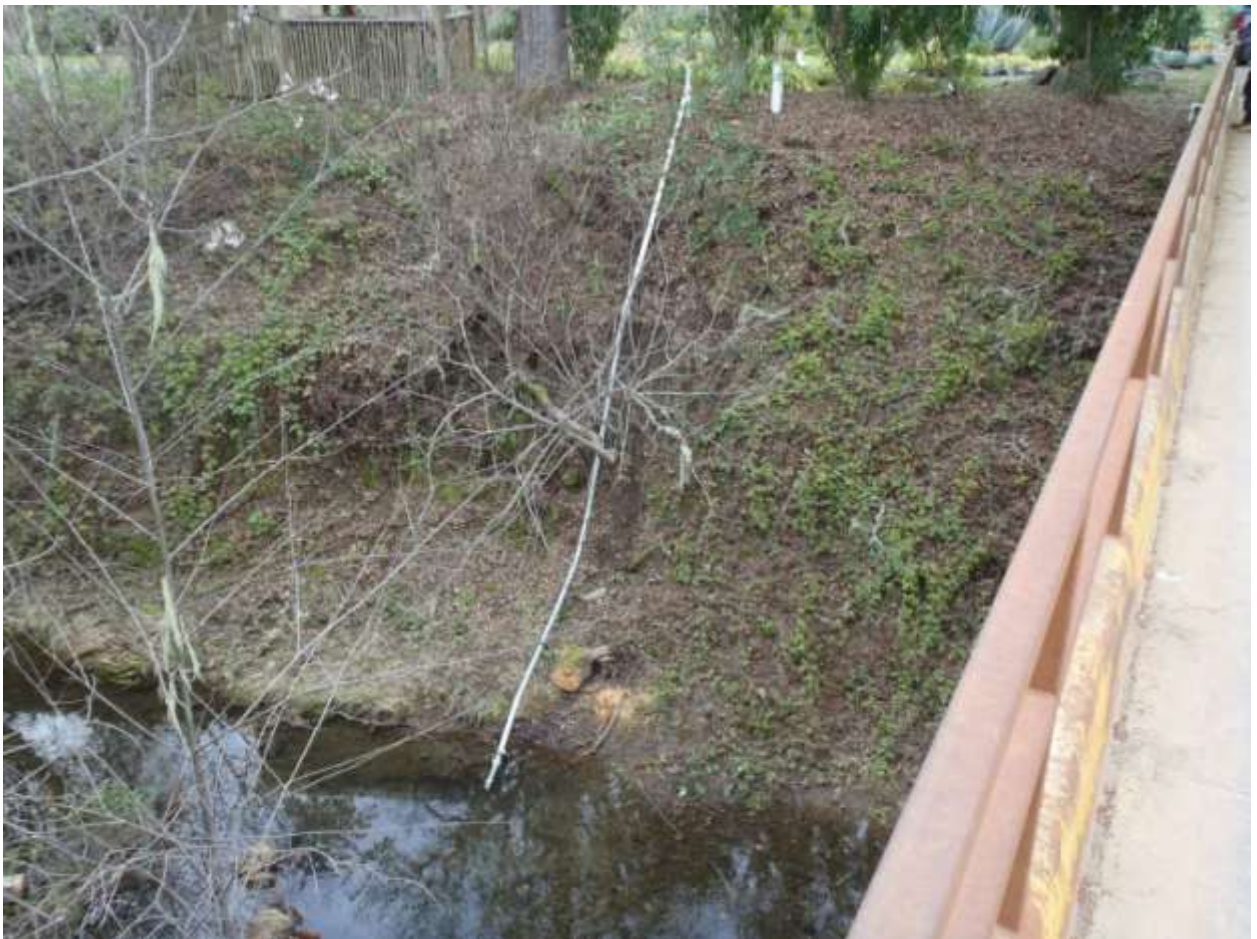
Figure 11: Example of a differential-pressure transducer. Note the cable extended above the transducer . Gage installed in pipe along stream bank.
