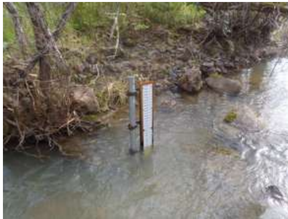
Figure 5b. Staff gage Installed in the McNab Creek Watershed
