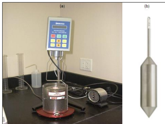
Fig. 3.9. Viscosity measurement apparatus: (a) Brookfield -II+ Pro viscometer, and (b) Spindle.
