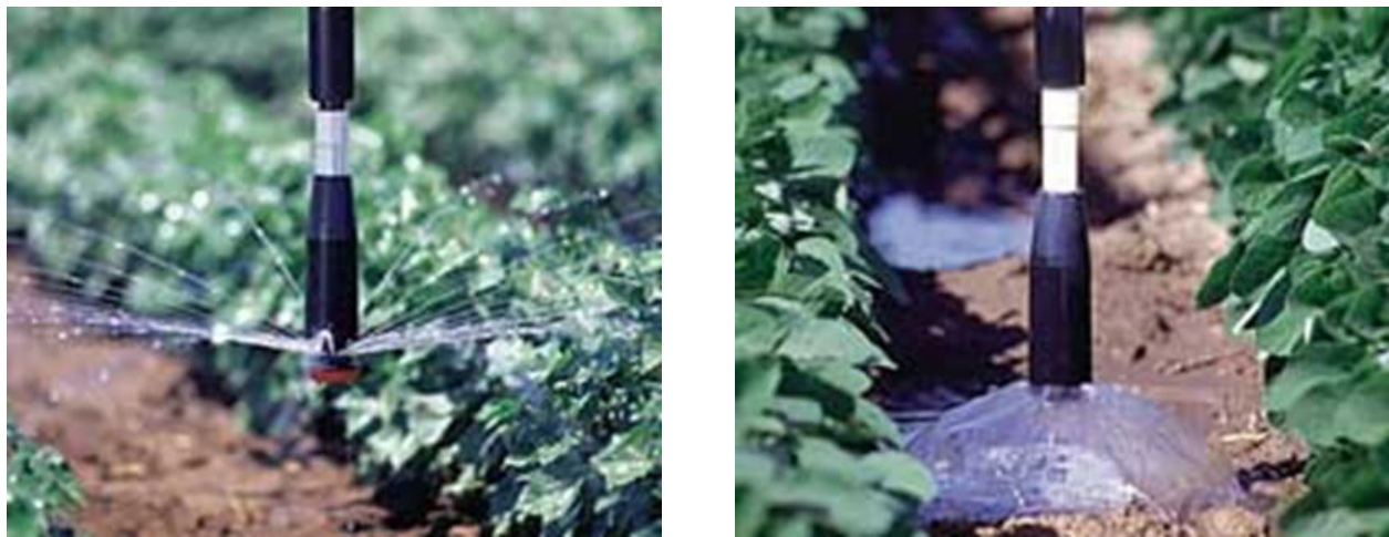
Figure 12: Photos of the Spray (Left) and Bubble (Right) Modes of the LEPA System.
