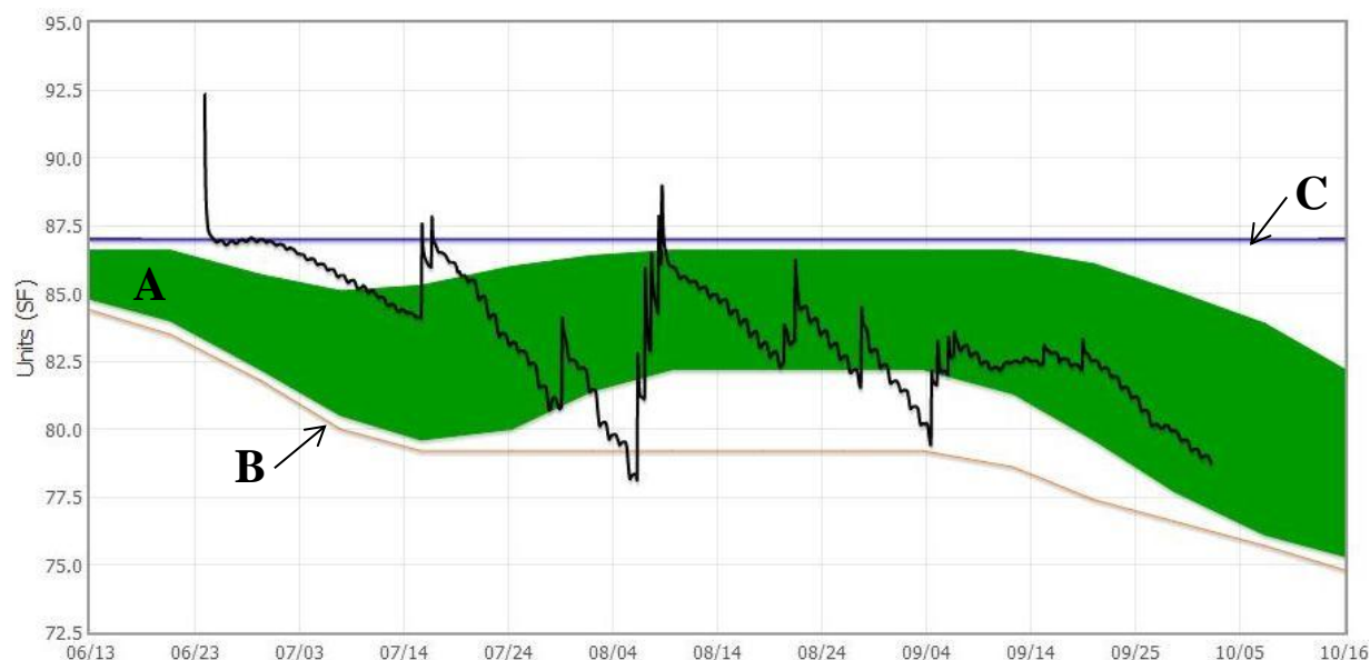
Figure 5: The summary graph for all sensors in an AquaSpy™ Probe. A) The green area is the optimal level for the soil moisture for the crop. B) The red line represents the refill point. C) The blue line represents the field capacity for the soil.
