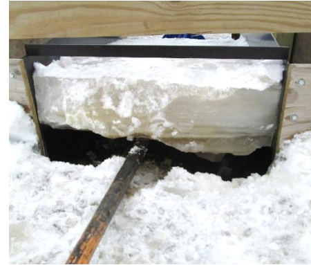
Figure 14. Thick ice easily removed after running the flume heater for ten minutes
