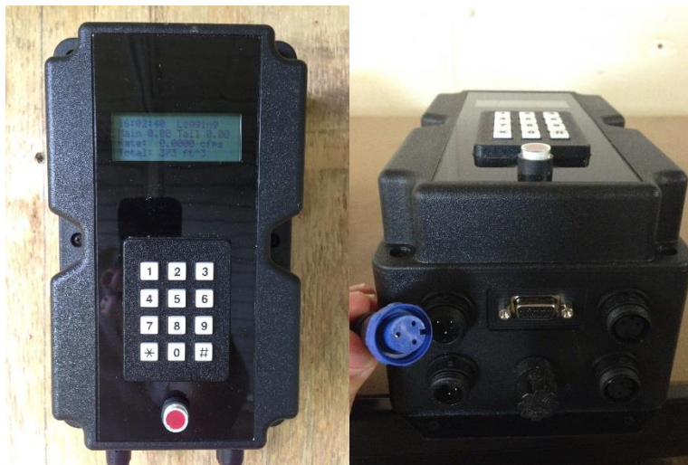
Figure 5. Second generation datalogger with lcd screen, keypad, and threaded cable connectors
