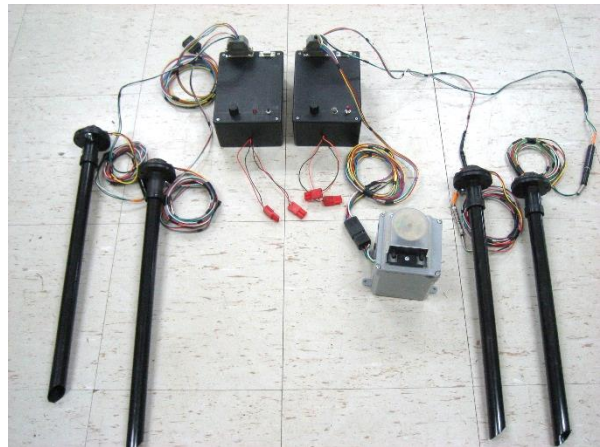
Figure 12. First generation electronics kit including primary and backup dataloggers and sensors, sample pump, and wiring harnesses
