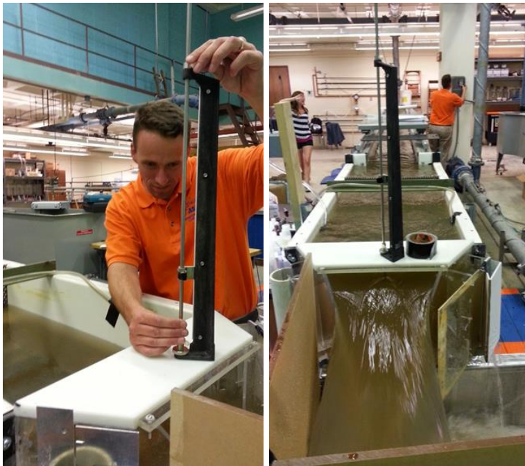
Figure 24. Point gauge measurement of water surface (left), h flume and approach during high flow trial (right)
