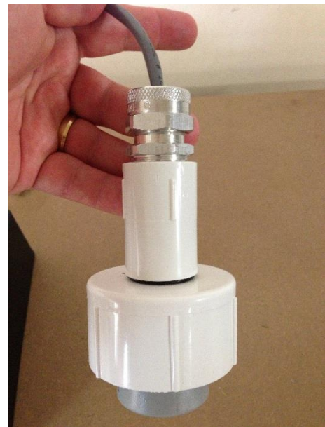
Figure 3. Sensor with custom weather proof housing
