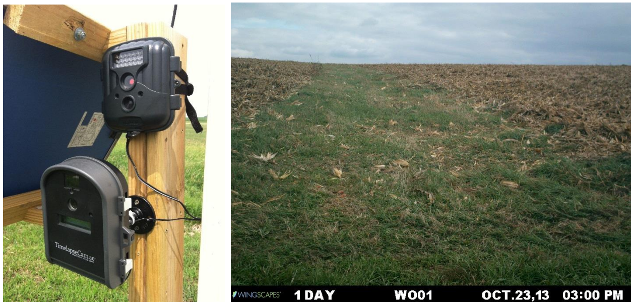
Figure 8. Timelapse and motion triggered trail camera (left). Sample timelapse image (right).
