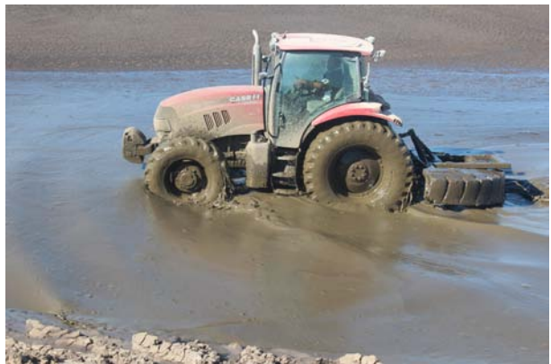
A tractor with a rear-mounted tire pushes manure to the lagoon pump
