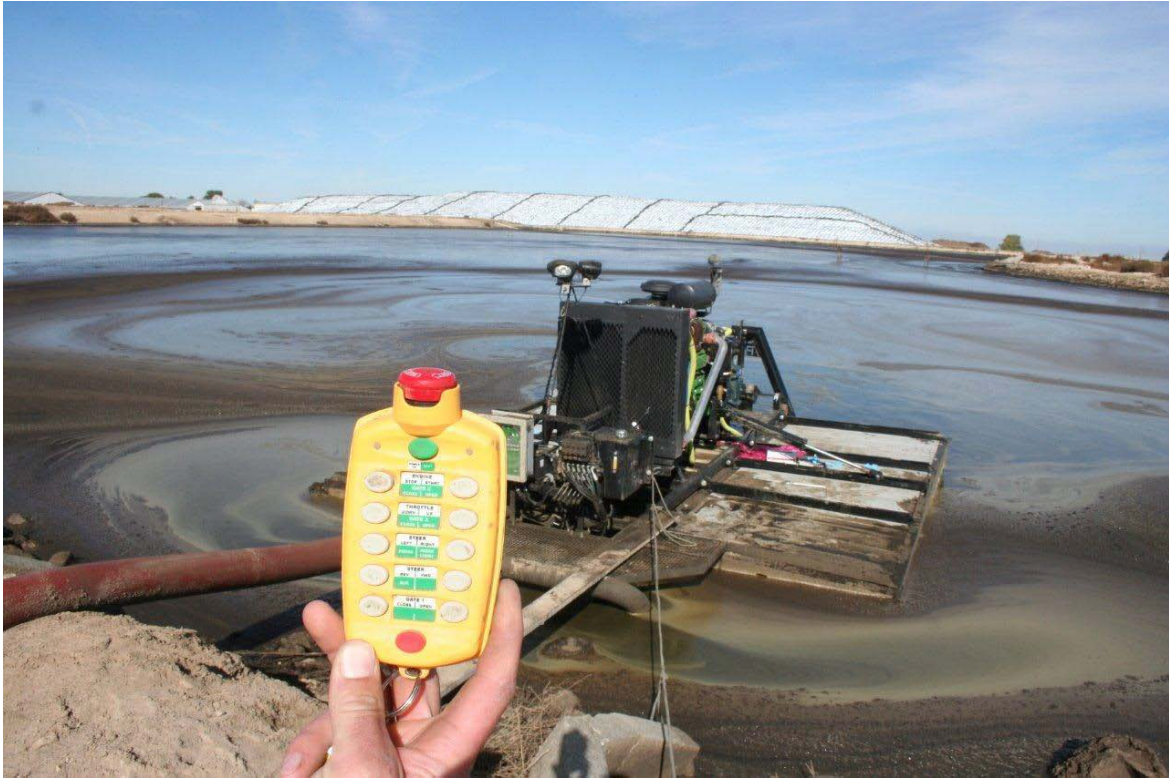
A floating mixing pump and a remote controller (yellow)
