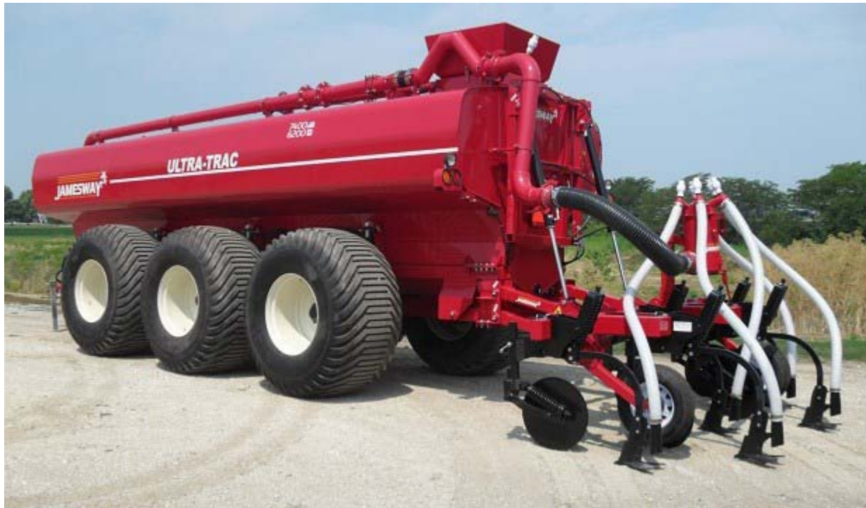
Subsurface manure injector with a manure tank
