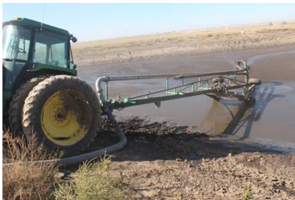
A lagoon mixer driven by a tractor
