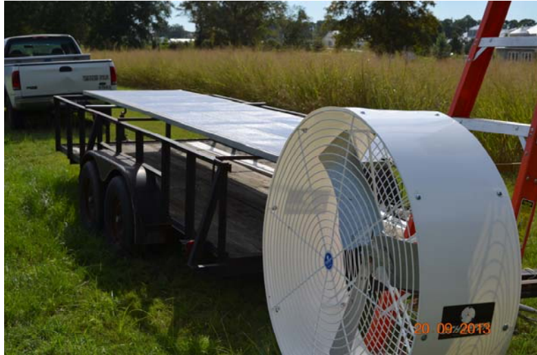
Figures 2(a) and 2(b). These are images of the solar fan on display. A can be seen the fan is run directly from the solar panels.
