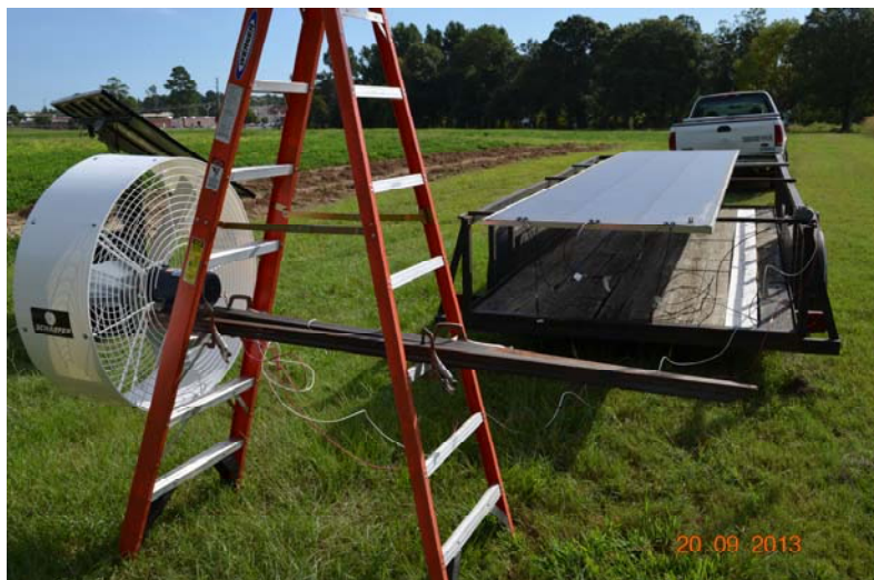
Figures 2(a) and 2(b). These are images of the solar fan on display. A can be seen the fan is run directly from the solar panels.
