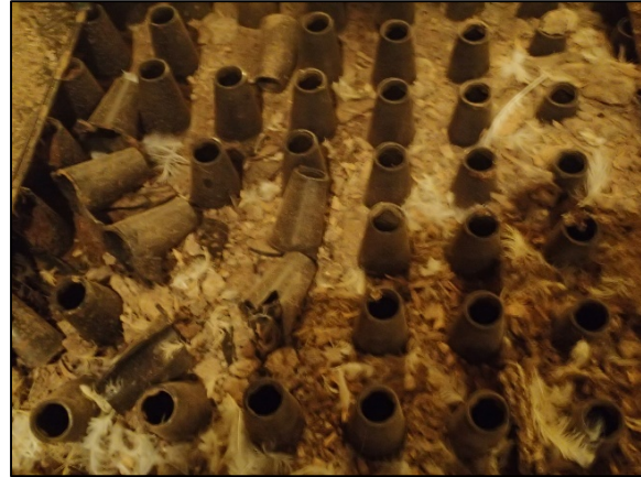
Picture 12. Damaged support cones
