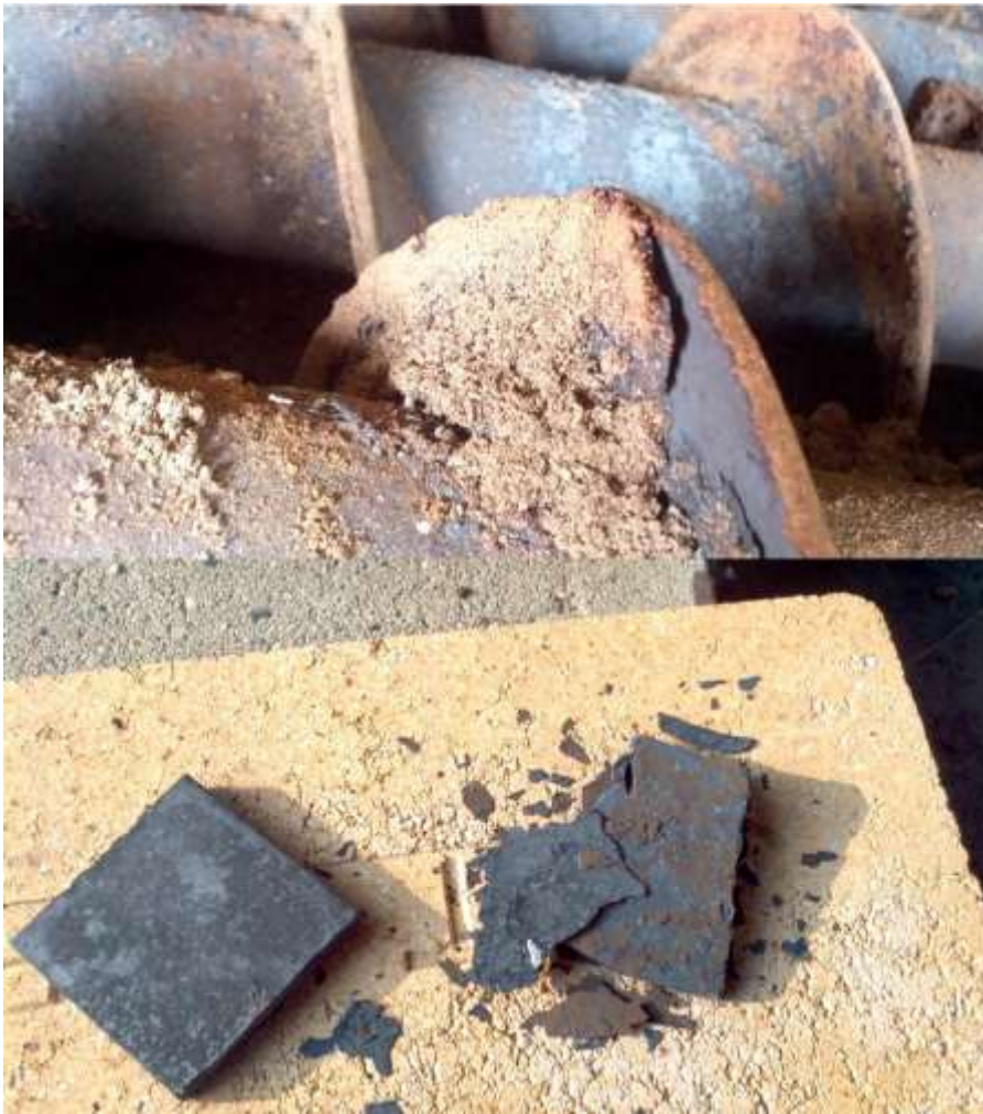
Top: damaged auger in 6-auger gasifier Bottom: 309 vs 304 muffle furnace test
