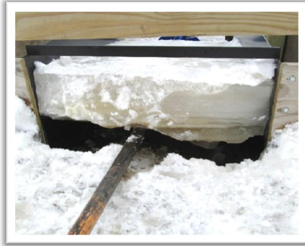
Figure 5. Thick ice easily removed after running the flume heater for ten minutes.
