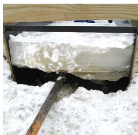
Figure 5. Ice is easily removed from flumes with integrated hydronic heat systems.
