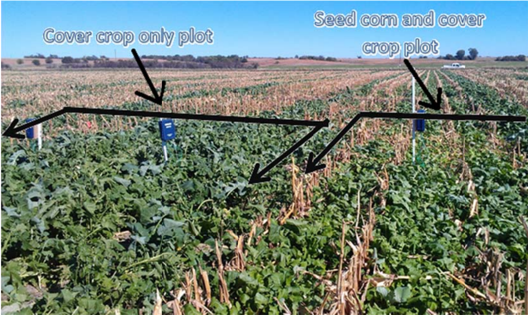
Picture 18. Three fields have a four-plot Watermark sensor set-up for measuring the differences in soil water between plots of (1) cover crop only, (2) seed corn and cover crop, (3) seed corn only (not pictured), and (4) bare soil (not pictured). This picture is of a primarily turnip mix in fall 2013.
