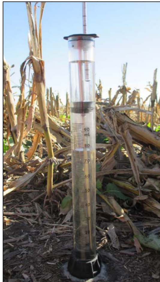
Figure 22. Mini Disk Infiltrometer for estimation of unsaturated hydraulic conductivity K(h) .
