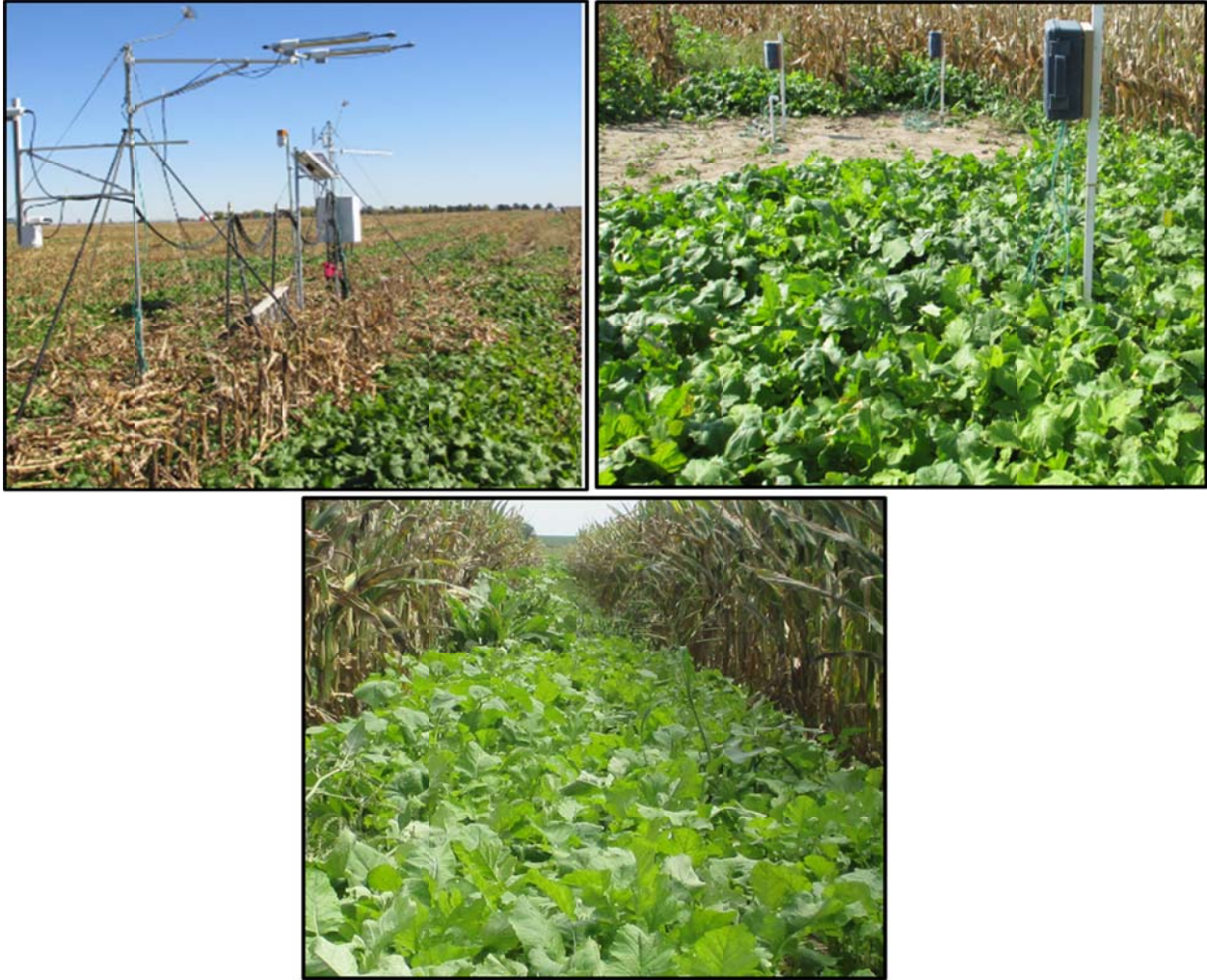
Figure 2. Bowen Ratio Energy Balance System (BREBS) at the F1 field and different treatments in seed maize-cover crop rotation fields.
