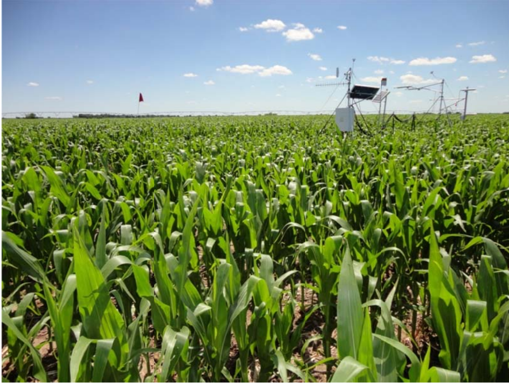
Picture 15. The Bowen ratio energy balance system (BREBS) installed at the primary site records hourly water balance, energy balance, and microclimate parameters year-round.
