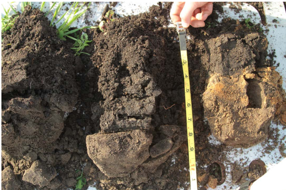
Figure 5: Soil Profiles of 6a, 6b and 6c (left to right) taken on November 2012. Note the platy soil structure (as a result of compaction by traffic) already begins at 3”- 4” in this image.
