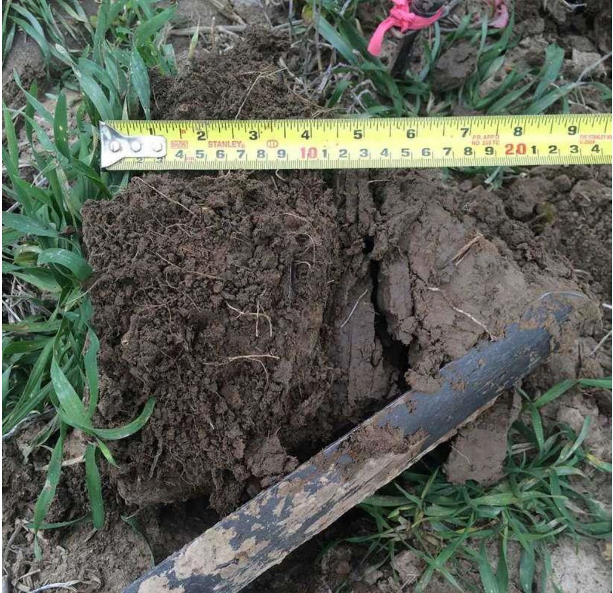
The compacted layer in this conventionally tilled field clearly begins at 4.5 inches.
